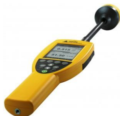
Fig. 4.2. The meter of electromagnetic field voltage (Narda NBM-550).
