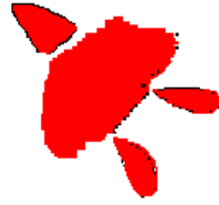
Fig.4. Occurrence of petals of a distorted beam of the laser
